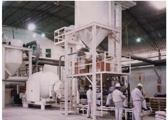
Workers package insecticide after it has been mixed by the rotary mixer
