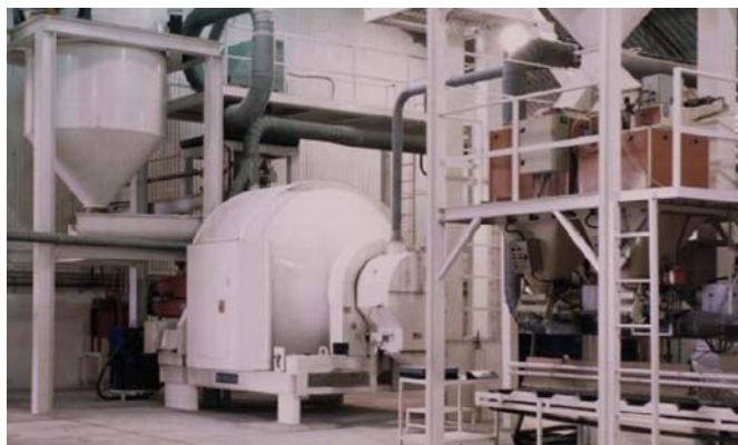
The hopper (on the left) feeds clay or quartz into the 700-TSC-180 rotary mixer. Chemicals are sprayed as the batch rotates
